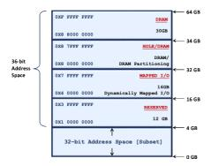
Using 36 bits (address bus), we can design a 64-bit SoC comfortably with all I/O interfaces, controllers, and memories within a 64GB address space. This allows us to expand the DRAM more than 30 to 40 GB and realize any kind of bare-metal complex embedded and OS-based desktop applications.
